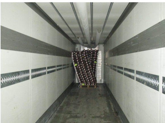
Pallets deformation in front part of refrigerator-trailers
