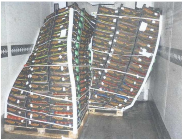
Pallets deformation in front part of refrigerator-trailers
